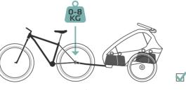
An optimal tow bar load ensures a safe driving behavior.
