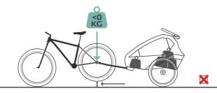
A too low tow bar load can push the bike upwards.
