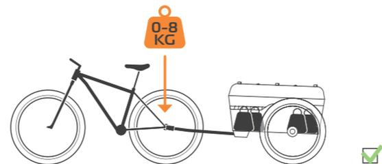
An **optimal** tow bar load ensures a safe driving behavior.
